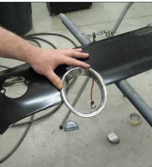
We kept test fitting the surround until they slid in-to place with ease. This can take some time as you are making custom holes.
