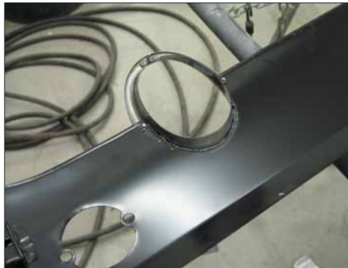
Though you can't see it here, the outer edge of the new National Parts Depot surround is gapping at the intersection of the lip and the curve of the panel. The yellow dots are there to remind us what needs to be removed with the cutoff wheel so the panel will seat.
