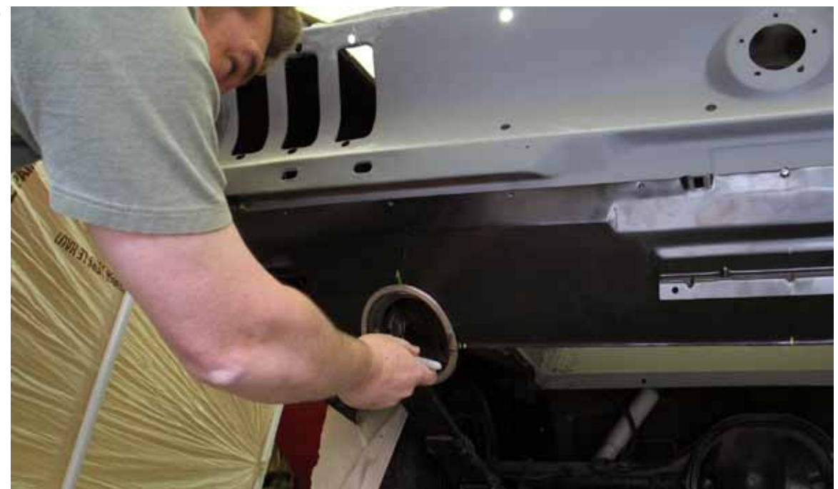
We then installed the panel and eyeballed the angle needed for the surround's inside cuts. Had we done this off of the car we would have badly misjudged the cut.
