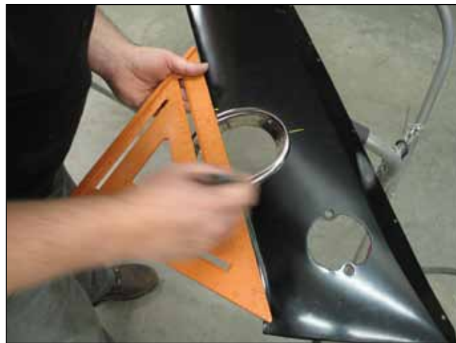
We used a speed square (all we needed was a straight edge and it was handy) to set our line on the surrounds relative to the bottom edge of the valance. Be sure to do this after the surrounds are in place. If you do it first you are sure to cut them wrong.
