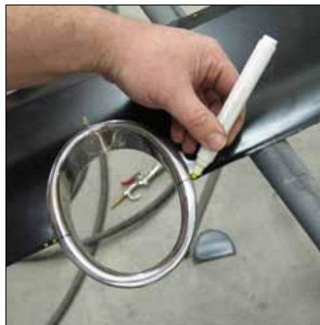
We used our paint pen to mark the edge of the new NPD surround so we can notch the panel. Make sure if you do this to notch jut inside the mark not on the line.
